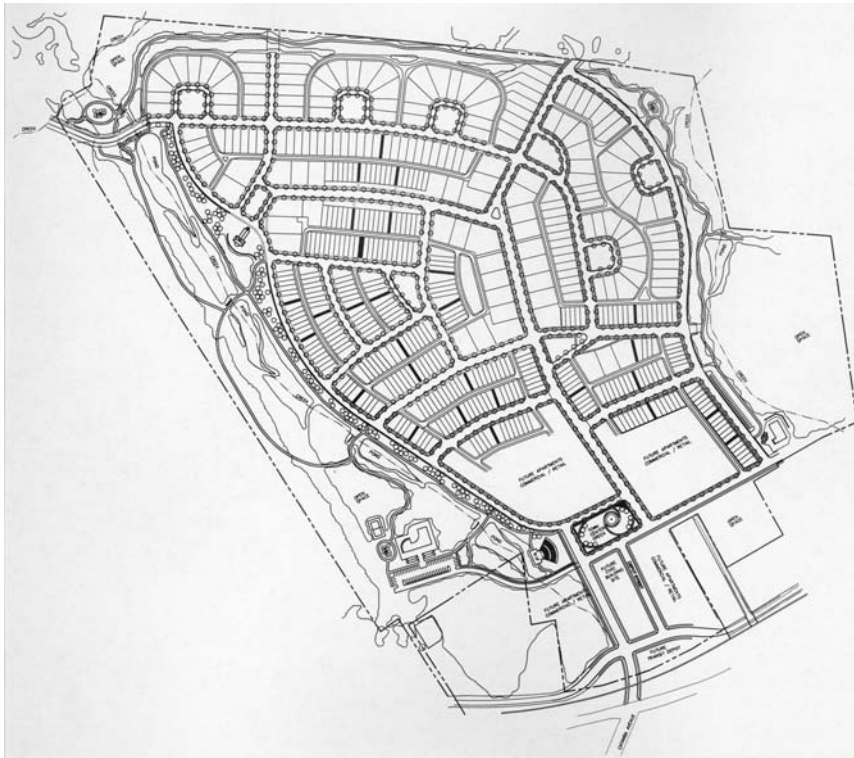
Figure 11.7 Revised TOD Master Plan Layout, Cole Jenest and Stone, Landscape Architects, 2001. This plan retained many elements of the original DPZ plan, but revised parts of the street pattern to suit detailed topographical conditions. The commuter rail line makes a shallow arc on the left-hand edge of the drawing, and the train station will be located next to the pedestrian connection across the tracks to the adjacent town center. The mixed-use development discussed in this chapter is immediately off the drawing on the left-hand side. (Drawing courtesy of Cole Jenest and Stone)
